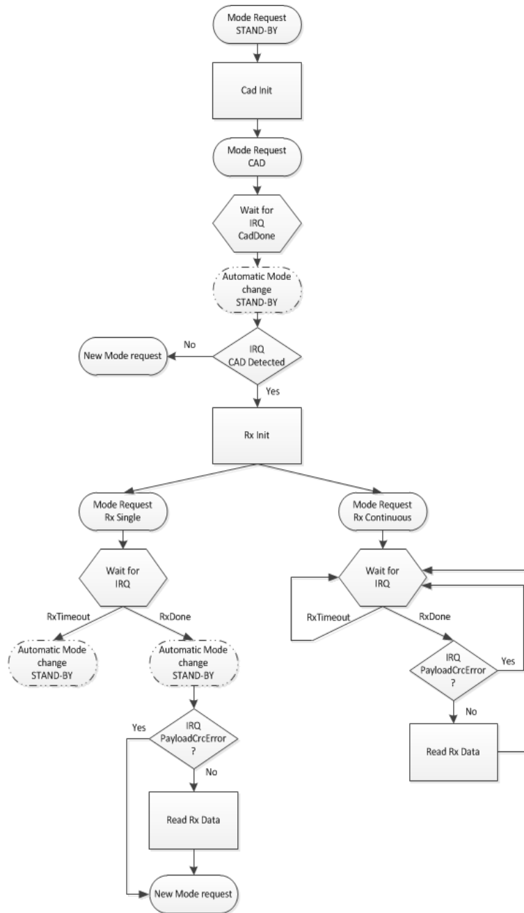
Figure 10. LoRa™ CAD flow
