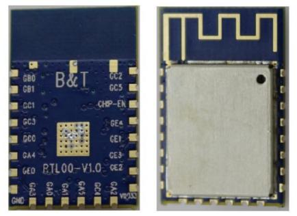
Figure 3 RTL00 module appearance
