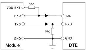
Figure 22: Level converting by diodes
