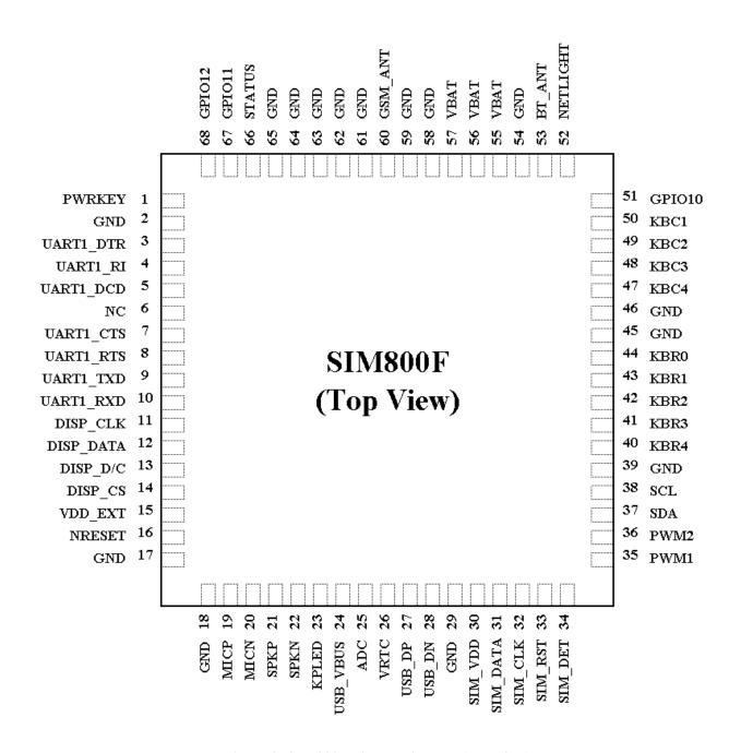
Figure 2: SIM800F pin out diagram (Top view)
