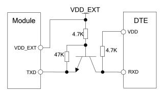
Figure 23: TX level converting by transistor
