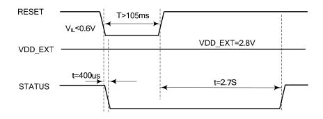
Figure 16: Reset timing
