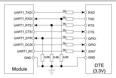
Figure 21: Level converting by resistor
