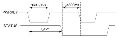
Figure 14: Timing of restart SIM800F
