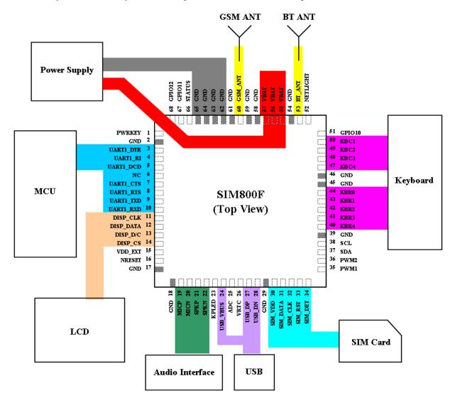
Figure 45: Pin assignment
