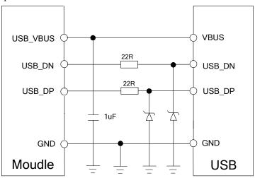
Figure 25: USB reference circuit
