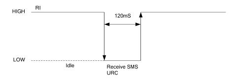
Figure 28: RI behaviour of URC or receive SMS
