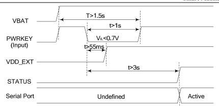
Figure 12: Timing of power on module
