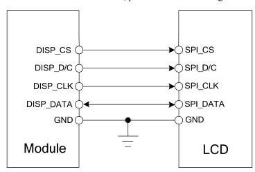
Figure 36: Connection of DISP interface
