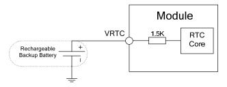
Figure 19: RTC supply from rechargeable battery
