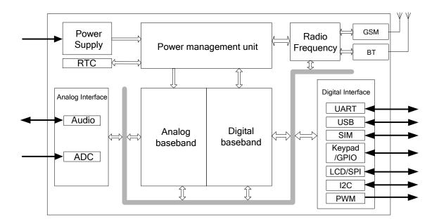
Figure 1: SIM800F functional diagram
