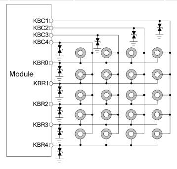
Figure 37: Reference circuit of the keypad interface
