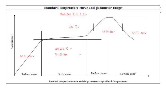
Figure 47: Typical Solder Reflow Profile
