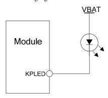
Figure 41: KPLED driver reference circuit
