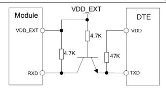
Figure 24: RX level converting by transistor
