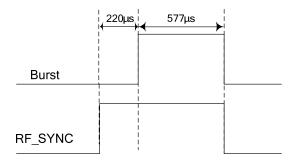
Figure 38: RF\_SYNC signal during transmit burst
