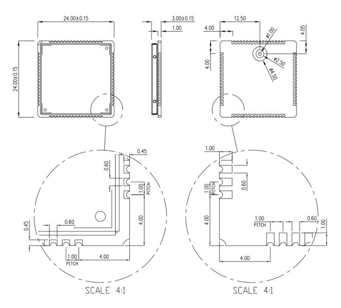
Figure 3: Dimensions of SIM800F (Unit: mm)
