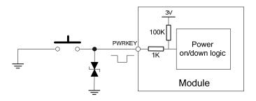
Figure 11: Powered on/down module using button
