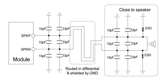
Figure 30: Speaker reference circuit
