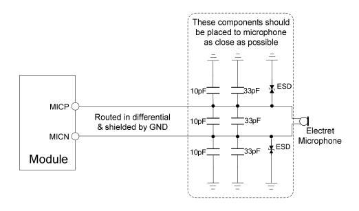
Figure 31 : Microphone reference circuit
