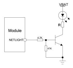
Figure 39: Reference circuit of NETLIGHT
