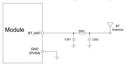
Figure 44: Bluetooth antenna matching circuit
