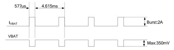
Figure 8: VBAT voltage drop during max power transmitting
