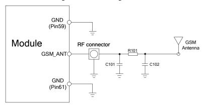
Figure 42: GSM antenna matching circuit
