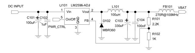
Figure 6: Reference circuit of the DC-DC power supply
