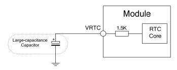
Figure 17: RTC supply from capacitor
