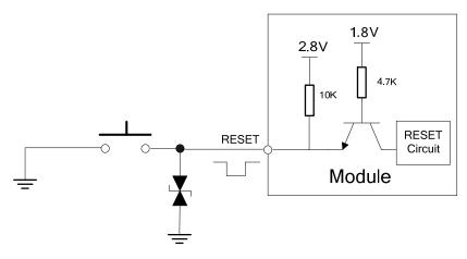
Figure 15: Reset Circuit
