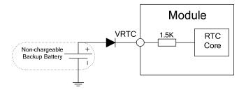
Figure 18: RTC supply from non-chargeable battery
