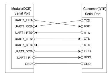
Figure 20: Connection of the serial interfaces
