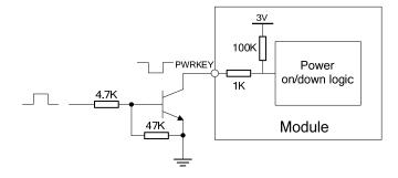
Figure 10: Powered on/down module using transistor
