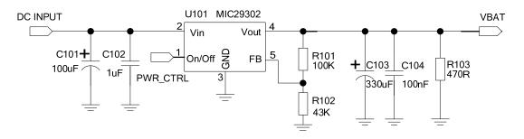
Figure 5: Reference circuit of the LDO power supply
