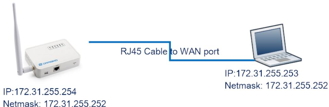
The LIG16 has a fallback ip in its WAN port. This IP is always enabled so user can use fall back ip to access LIG16 no matter what the WiFi IP is. The fall back ip is useful for connect and debug the unit.
